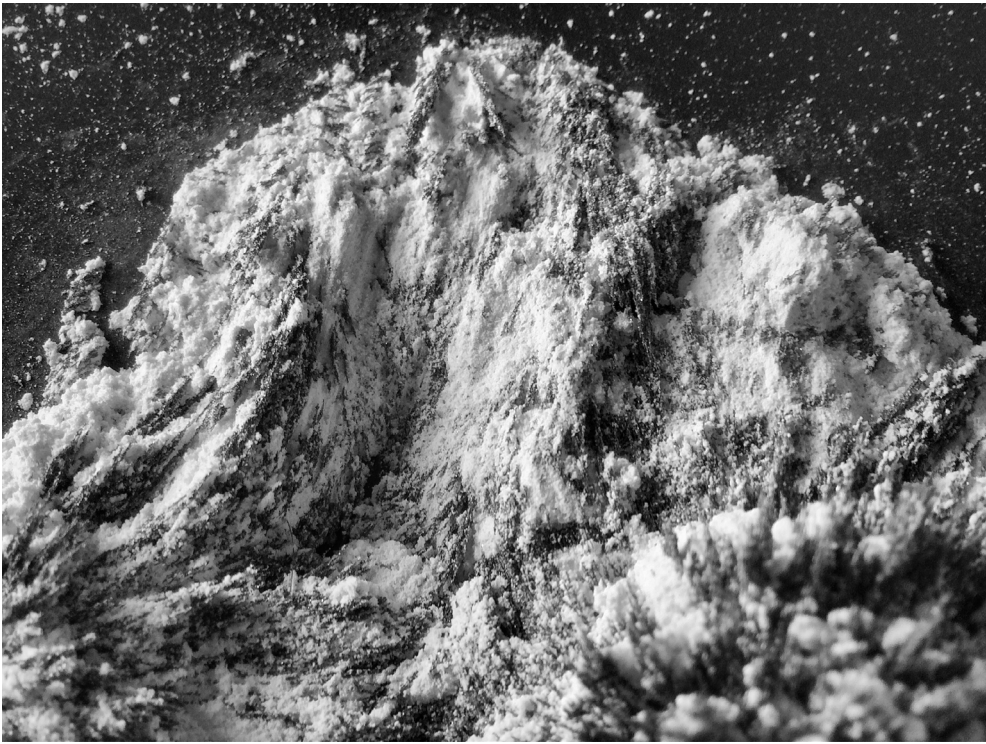
FIG. 25: IN-BETWEEN SORTING MATTERS OF THE MENTIONED PROCESS (FIG. 24) (SILICA SAND AND IRON POWDER)
