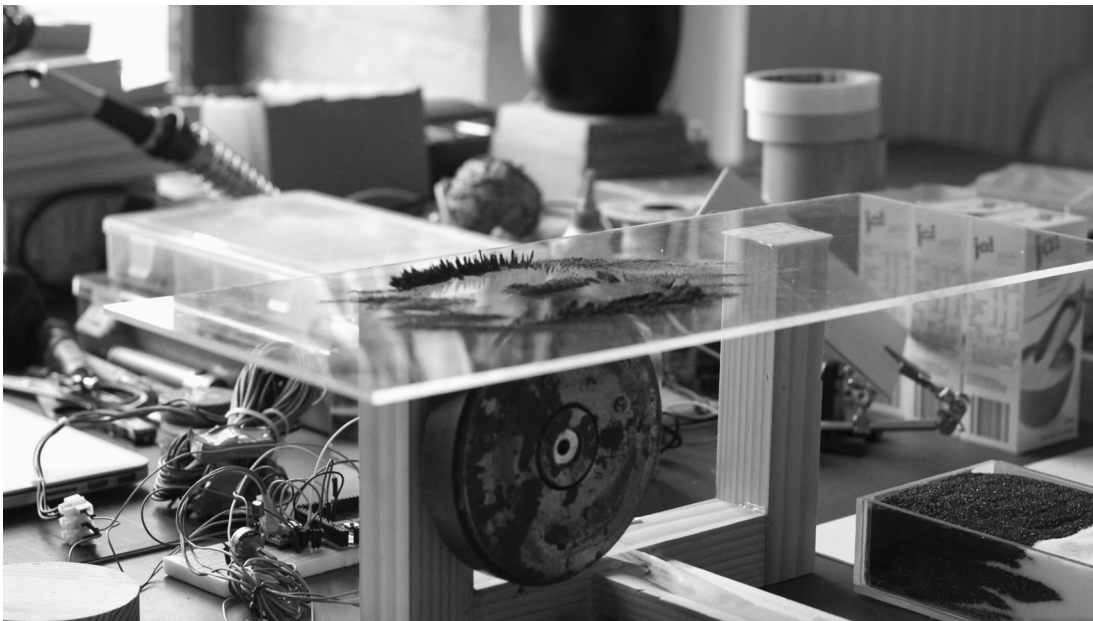
FIG. 23: EXPERIMENT WITH A MAGNET ATTACHED TO MOTOR AND PLATE WITH IRON POWDER
