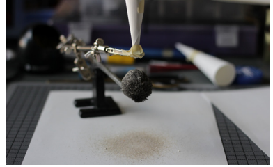
Experiment: sorting sand with magnet
